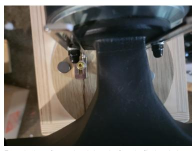
Face the horn forward and align the front lip flush with the baffle. Secure using the outer screws and washers (not the middle screw). Tighten just until snug - do not over-tighten.
