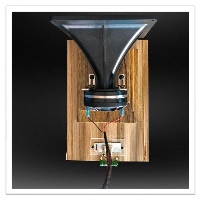
The horn assembly should be placed securely on top of the cabinet with the mouth of the horn facing forward. The lip of the horn should be located to line up with the font of the cabinet. Moving the horn forward and back on the cabinet top will subtly change the high and midrange frequency response.
